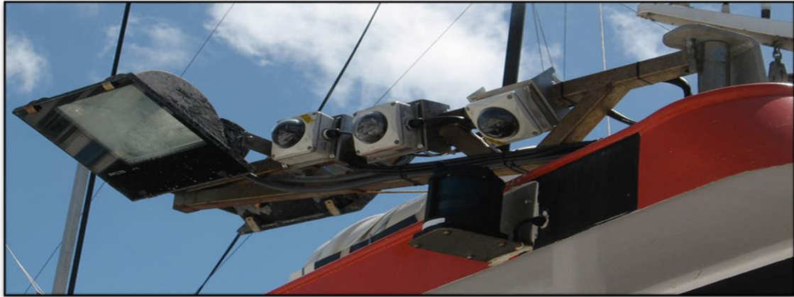
Photo: Example of electronic vessel monitoring to independently verify catch and monitor bycatch.
