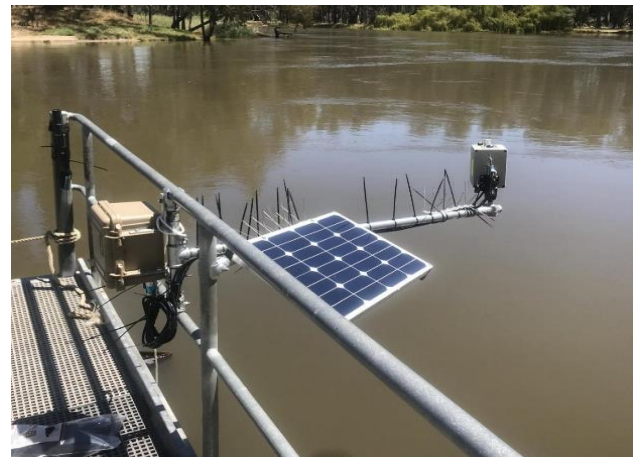
Water quality camera (HydraSpectra) deployed at, Barmah on the River Murray, Victoria. CSIRO.
