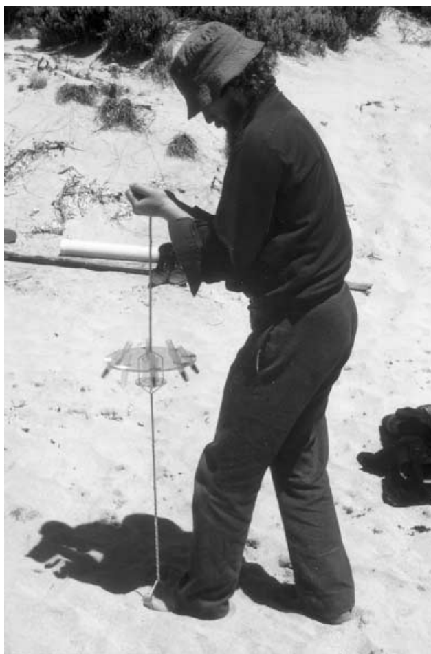
Figure 14.6 Blood samples can be separated into plasma and the cellular fraction by centrifugation. Robust, hand-operated devices can be very effective in field conditions. [Photo by T.D. Schwaner]
