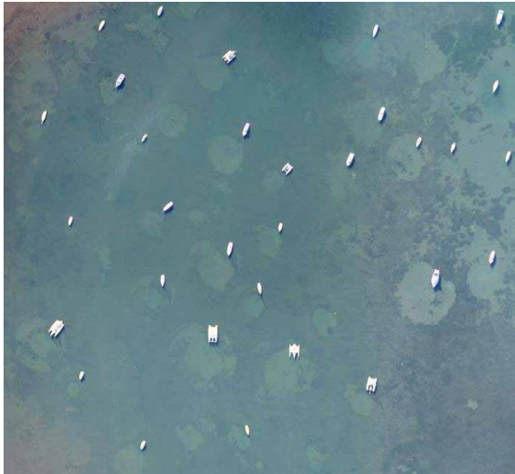
“Crop circles” caused by traditional moorings in Morton Bay (SEQ Catchments).
